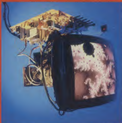
Dual scan monitors such as Commodore's 1942 have a limited frequency range, and thus are a cheaper buy.
